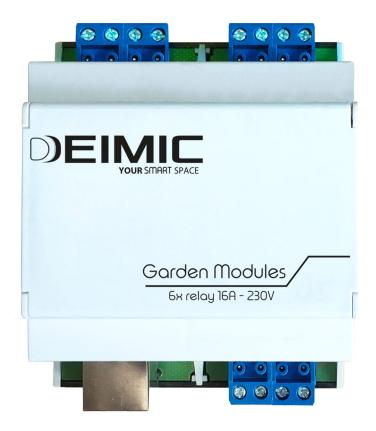
6x RELAY module is intended to use as external relays, which coils are powered with low voltage, so UTP cables can be used for controlling lights circuits.
